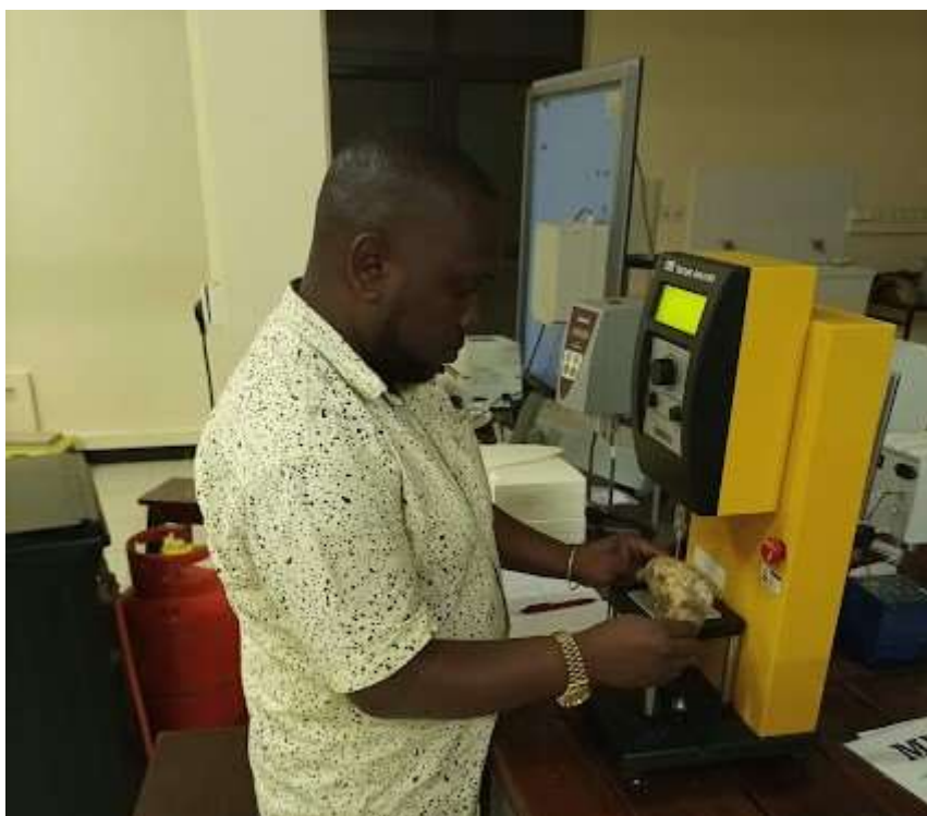
Plate 3.3: Hardness measuring by using a texture analyzer
