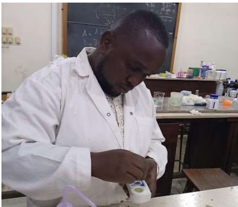
Plate 3.4: Total soluble solids measured by using Refractometer
