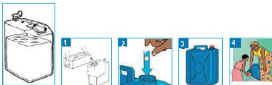
For clean water add 1 tablet in a 20 litre jerry can (filter the water through a clean cotton cloth if dirty). Wait 30 minutes before using.
