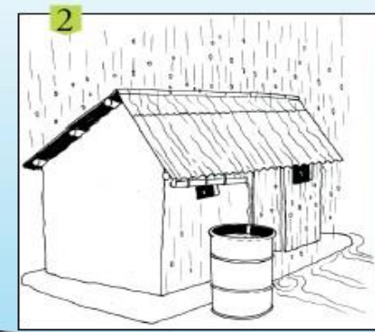
Rainwater harvesting without gutters
