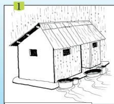
Rainwater harvesting without gutters
