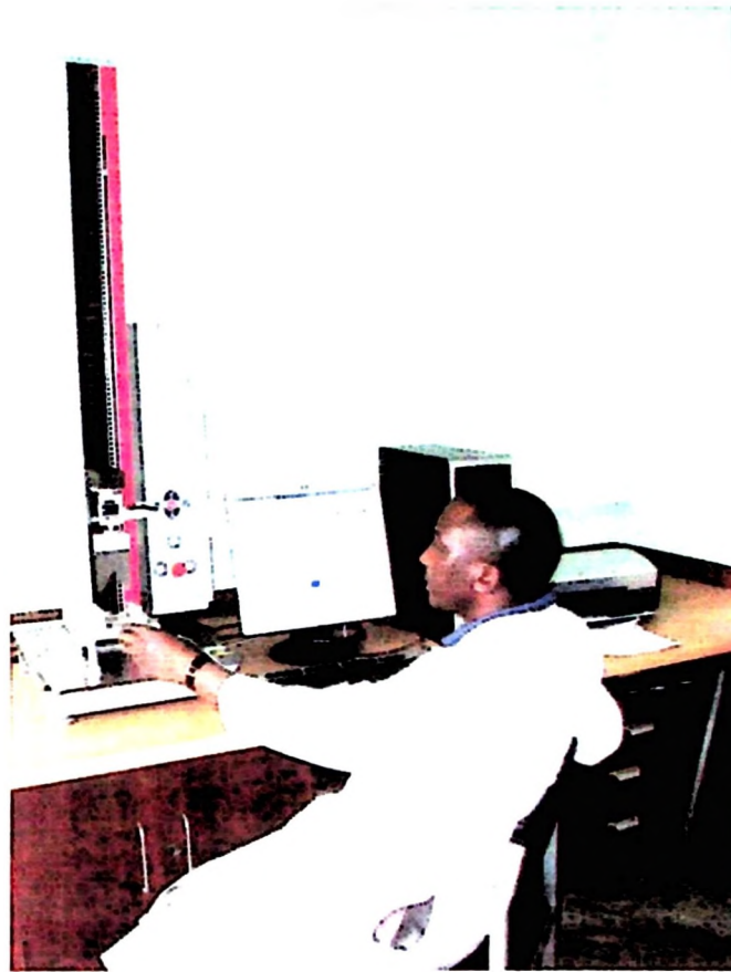
Plate 6: A researcher operating Warner-Bratzler Shear Force (WBSF) machine (Zwick/Roell Z2.5, Germany) for measuring meat tenderness
