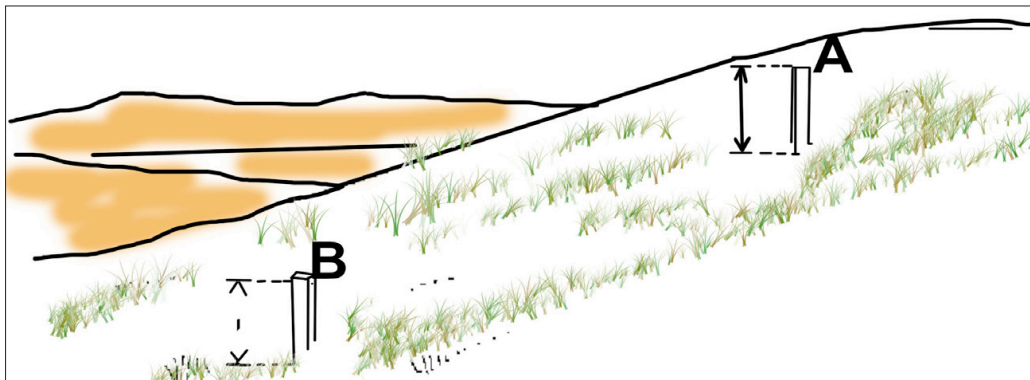
Figure 5.7. Measuring of horizontal distance and vertical on steep sloping areas
