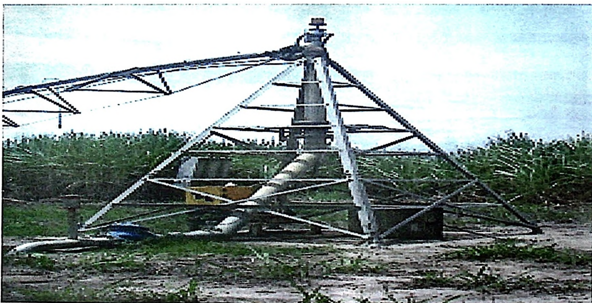
Plate 1: Pivot point of a centre pivot
