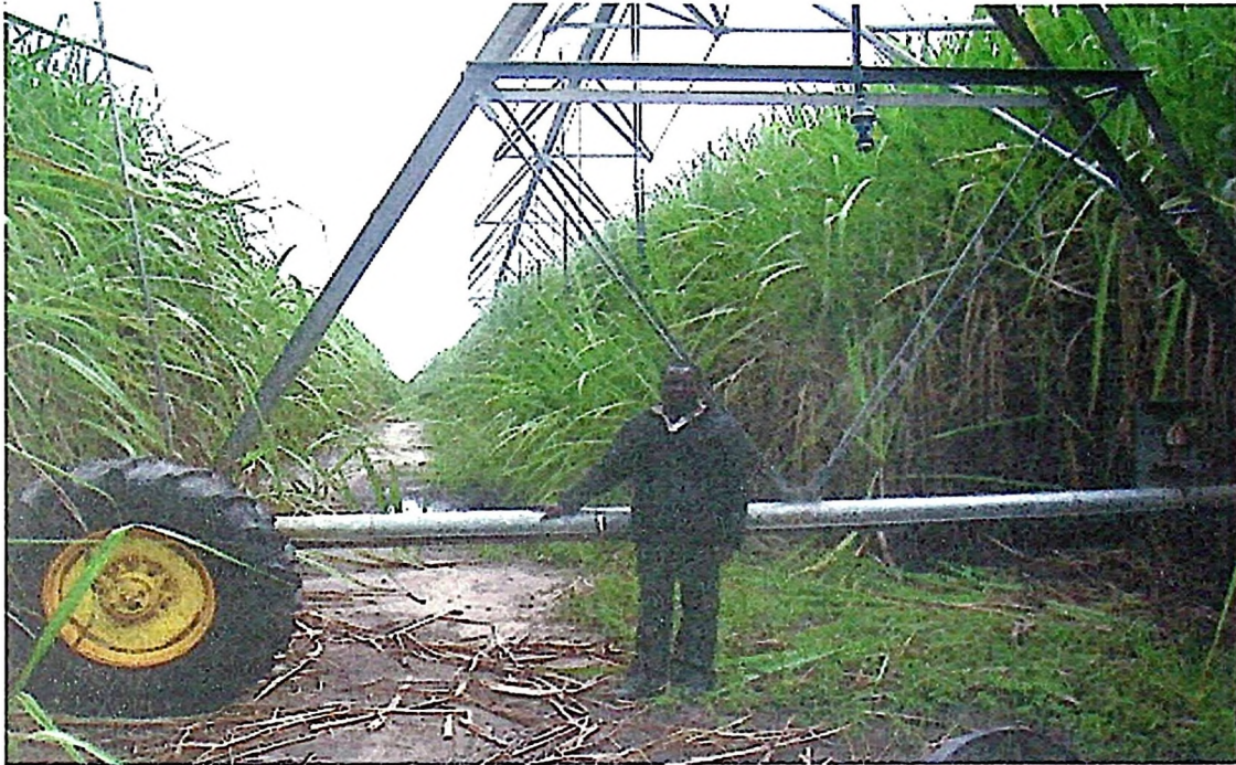
Plate 2: A-shaped steel frames (towers) mounted on powered wheels
