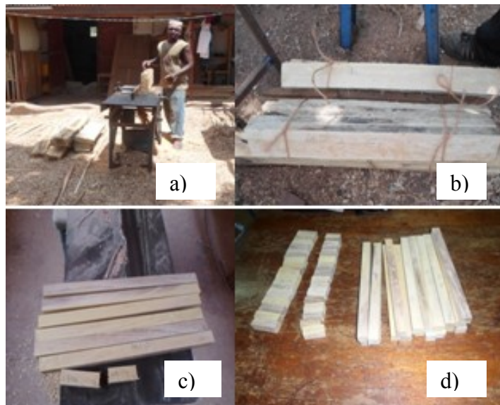
Figure 10: Sawing of cants and preparation of test specimens
