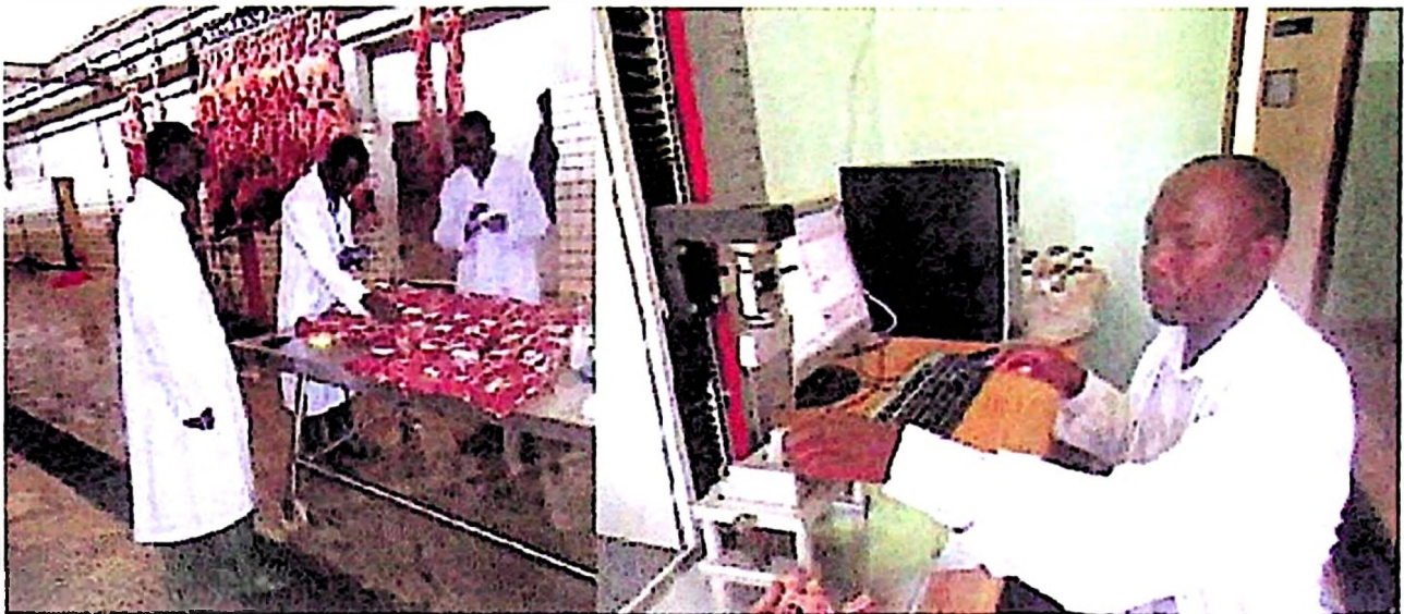
Figure 2: Measuring pH and tenderness of meat using a portable pH-meter and the Warner-Bratzler Shear Force (WBSF) machine respectively at DASP laboratory-SUA.
