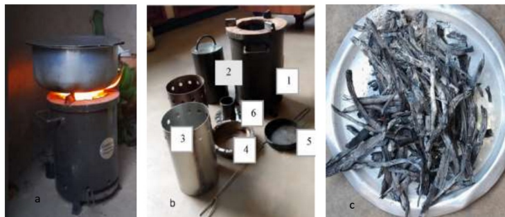
Figure 1. (a) Top Lit UpDraft gasifier stove. (b)stove parts: b1 =outer cylinder, b2 =extinguisher, b3 =inner fuel canister 4=top plate, b5 =ash collector, b6 =pelle
