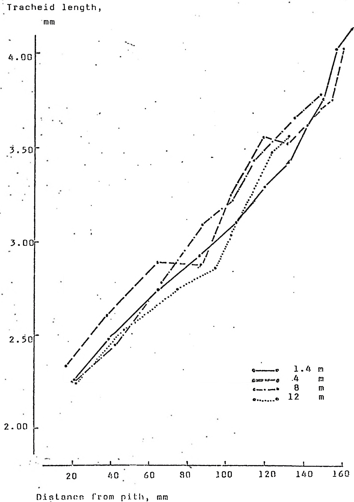
Figure 4.16 Relationship between latewood tracheid length and distance from pith at 4 heights in the stem.
