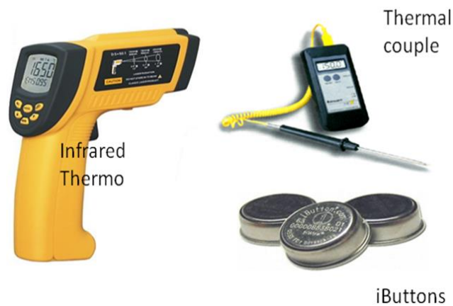
Figure 5.4: Equipment used to collect data for soil temperature and soil relative humidity
