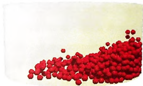
Figure 5.6(e) Particles forced up the cup wall reach the top of grain mass and roll/slide back t the dehulling disk
