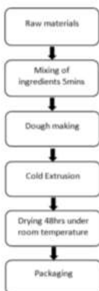
Fig. 4. A flow diagram showing noodle preparation Source: Modified from Orisa and Udofia, [18]
