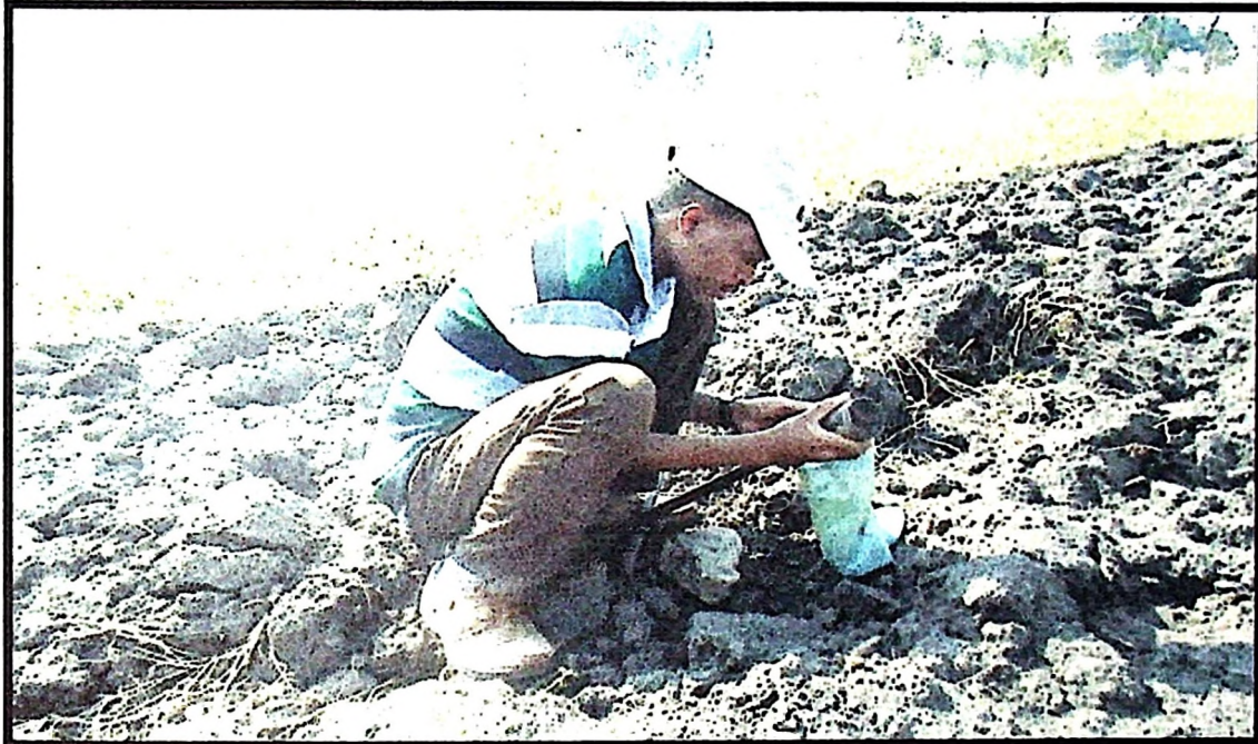
Plate 3.4 Collection of soil sample for bulk density measurement before operation
