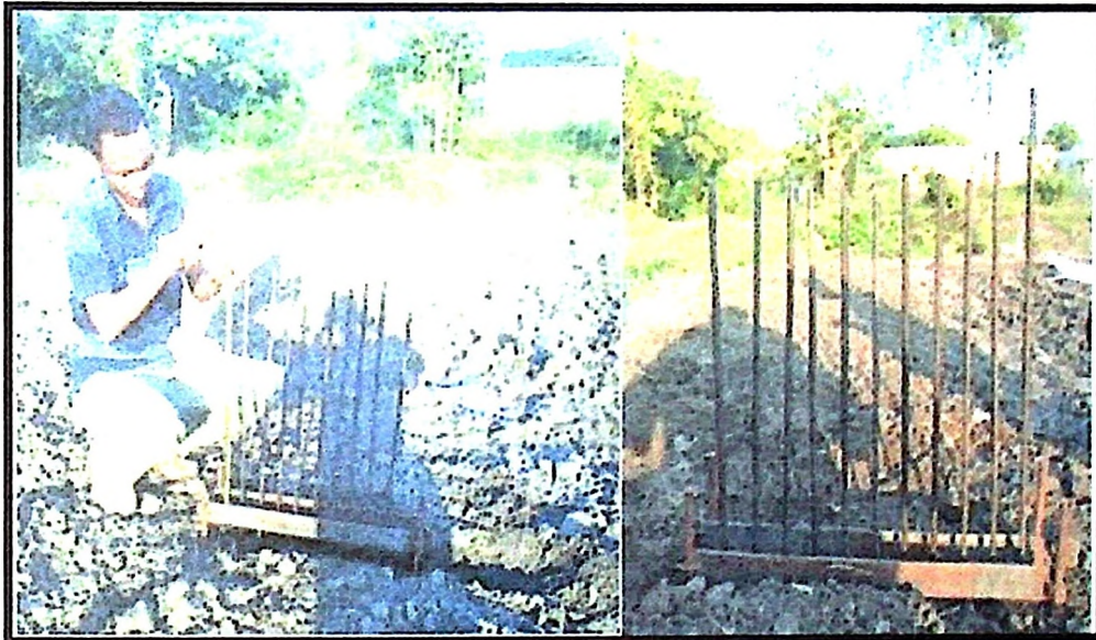
Plate 3.7 Measuring soil disturbed area by using soil profile meter
